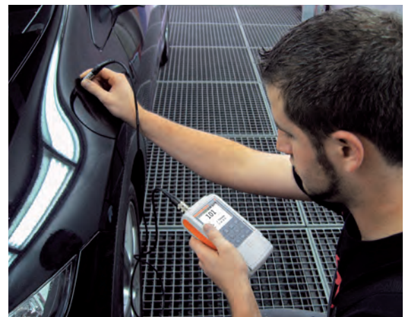
Paint coating thickness measurement using the dual probe FD13H
