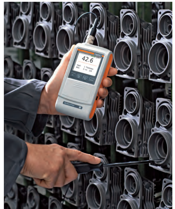
Measurements using the internal probe FAI 3.3-150
