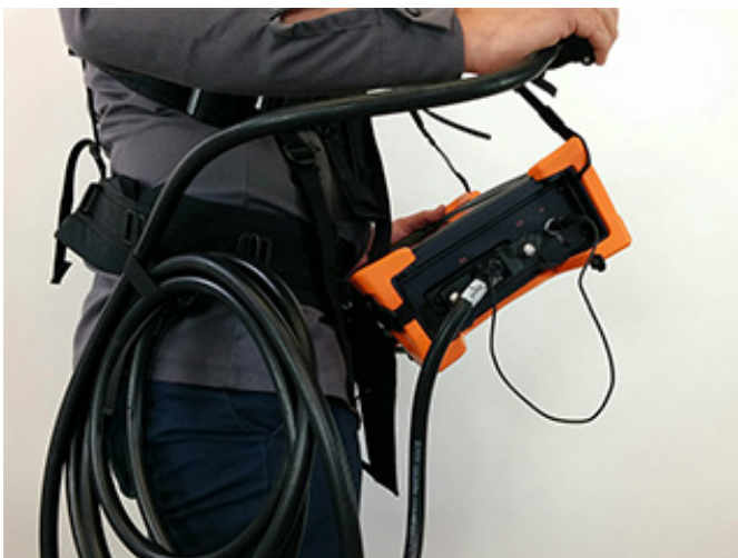
Figure B-17 Belt-slinging probe cable
