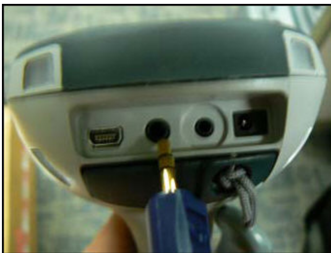
Figure 6. Plugging the Remote Trigger Cable Into the Analyzer
