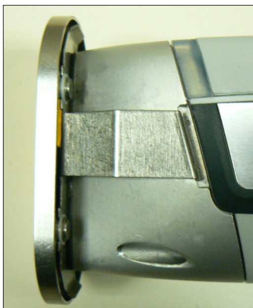
Figure 3. The In-Situ Test Guard in Place
