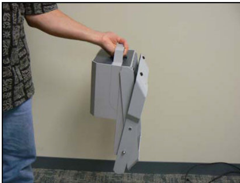
Figure 4. The Portable Test Stand Collapsed
