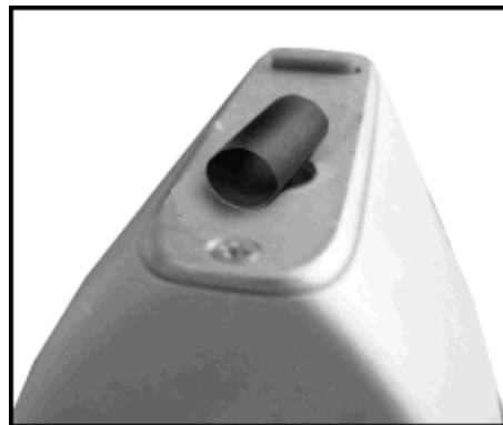
Figure 39. Incorrect Way to Measure Heat Shrink Tubing
